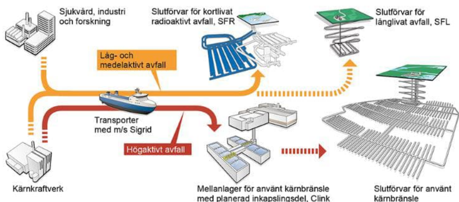
Figure 5. The existing system for managing radioactive waste and spent nuclear fuel. The blue rock chambers in SFR, the encapsulation facility adjacent to Clab and SFL, and the final repository for spent nuclear fuel are facilities that have yet to be built (Svensk Kärnbränslehantering AB).
